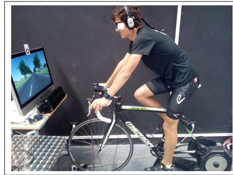
Figure 3: Experimental setup for cycling study with visual and auditory feedback with real-time animation of road-cycling experience (screen), visual feedback (handlebars), and sonification (headphones).
