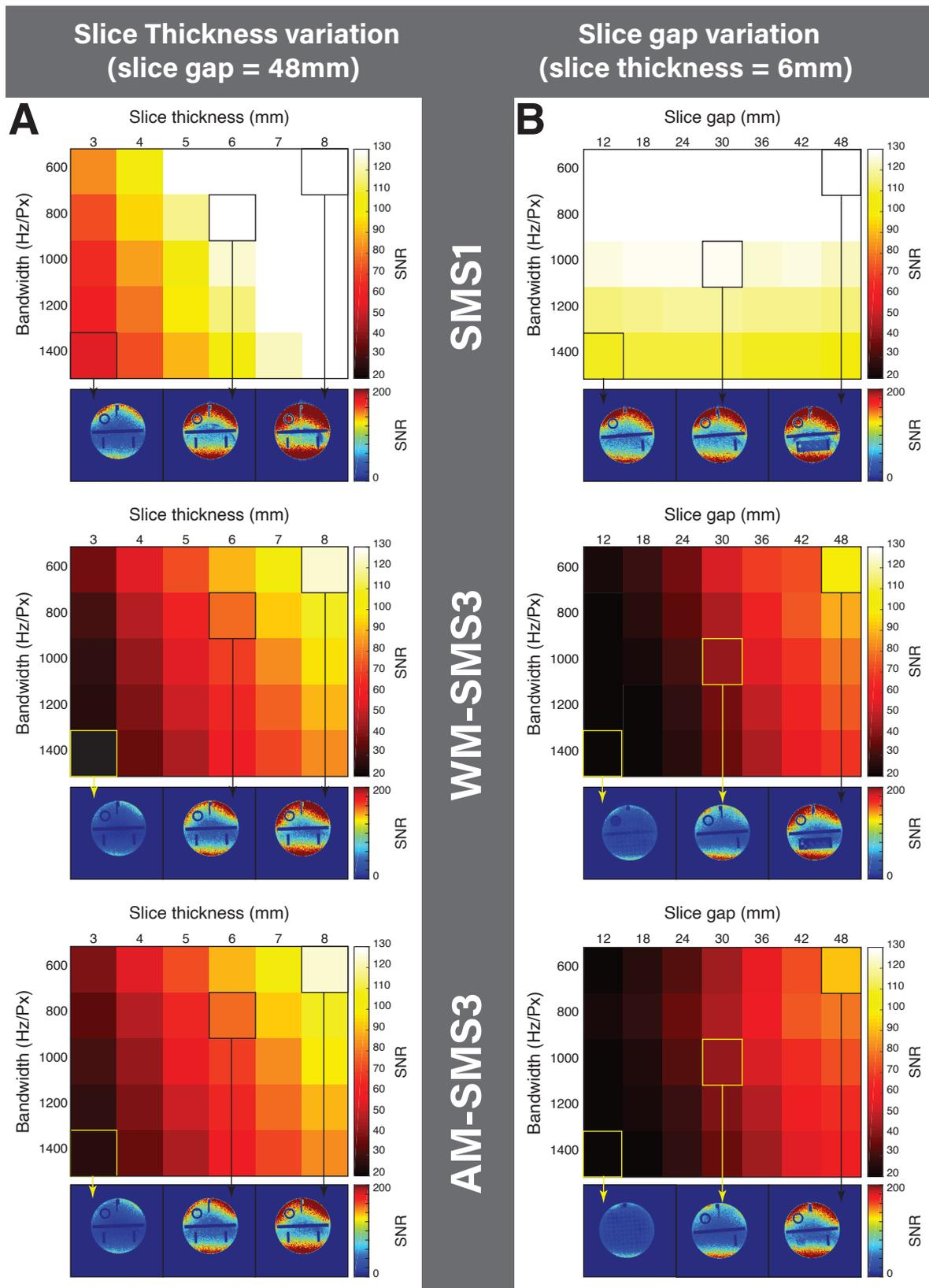
**Fig. 3.** SNR variation maps. (A): slice thickness and bandwidth variation (slice gap=48mm). (B): slice gap and bandwidth variation (slice thickness=6mm). Highest SNR values were obtained with higher slice thickness and slice gap, and lower bandwidth. WM, Wong modulation; AM, amplitude modulation.
