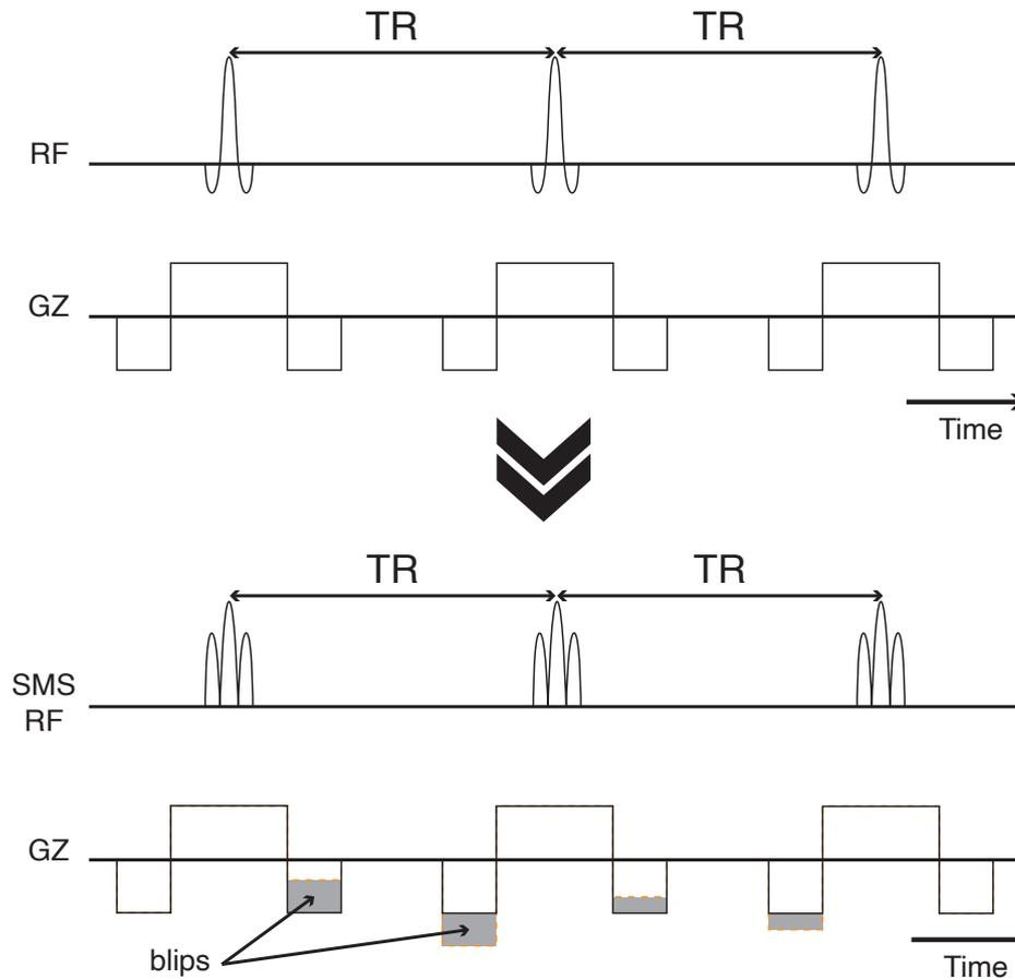
**Fig. 1.** Blipped CAIPIRINHA SMS-bSSFP. GZ Rewind gradients of the bSSFP are transformed into blips by adding and subtracting phase offsets at each TR. RF modulation is preserved, and bSSFP frequency response as well.
