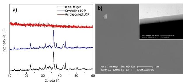
**Figure 1.** XRD patterns of the initial target, crystalline LCP film and as-deposited LCP film (a). Corresponding SEM images (b) of as-deposited LCP film from the top view and cross-sectional view (inset in Figure 1b).
