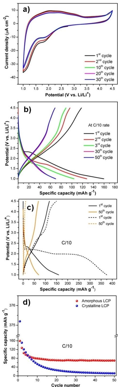
**Figure 2.** (a) Cyclic voltammograms of the as-deposited LCP film at a scan rate of 0.5 mV/s and (b) Typical galvanostatic charge/discharge profiles. (c) Charge/discharge profiles of (■) crystalline LCP film and (—) amorphous LCP film and (d) discharge capacity of the amorphous and crystalline LCP films at C/10.
