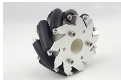
Fig. 1. Mecanum wheel design.
