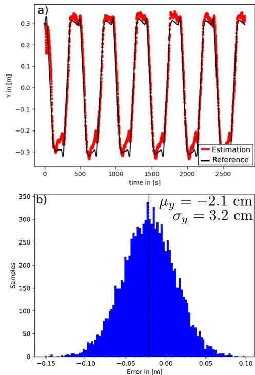
**FIGURE 16.** Estimation of position along y-axis. a) Comparison of the position estimation (in red) to the actual position of the robot (in black) versus time. b) Histogram of the localization error in 2D using In-Lock sensor.
