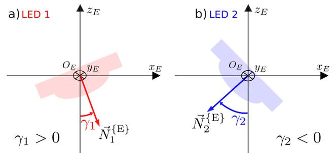
**FIGURE 6.** Illustration of the direction of emission of each LED with respect arbitrary angles  $\gamma_1$  for LED 1 (a) and  $\gamma_2$  for LED 2 (b).
