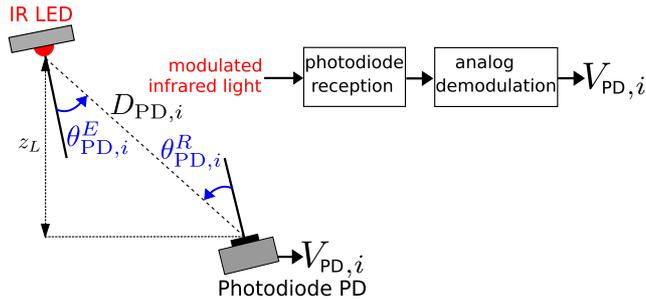
**FIGURE 4.** Side view of the optical wireless channel model. The model gives a nonlinear expression of the voltage amplitude  $V_{PD,i}$  for each frequency  $f_i$ . It depends on the angle of emission  $\theta_{PD,i}^E$ , the angle of reception  $\theta_{PD,i}^R$  and the distance  $D_{PD,i}$  from the beacon to the photodiode.
