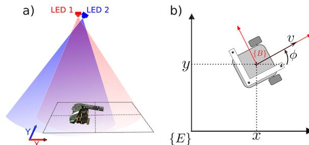
**FIGURE 1.** a) Perspective view of the sensing device. It is composed of 3 photodiodes (3 pixels) and a custom made analog demodulation board. It is embedded on the TurtleBot3 Burger for the experiments. b) Model of the mobile robot. The vehicle's body frame is shown in red and the earth frame of reference is shown in black. The velocity in the  $x$ -direction is  $v$  and the vehicle's heading is  $\phi$ .
