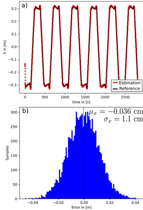
**FIGURE 15.** Estimation of position along x-axis. a) Comparison of the position estimation (in red) to the actual position of the robot (in black) versus time. b) Histogram of the localization error in 2D using In-Lock sensor.
