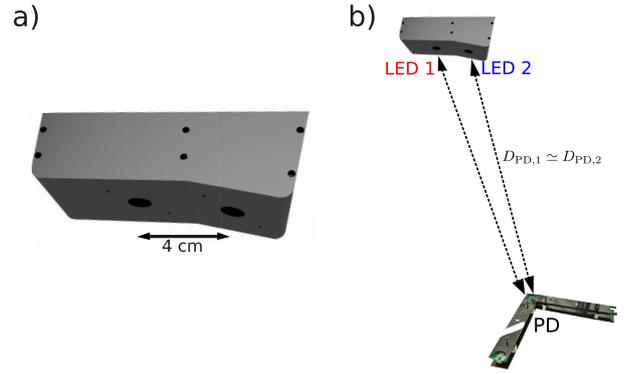
**FIGURE 5.** Computer Aided Design of the beacon. a) The distance between the LEDs is 4cm. b) Since the distance between the beacon and the receiver is greater than 3m, we assume that  $D_{PD,1} \simeq D_{PD,2}$ .
