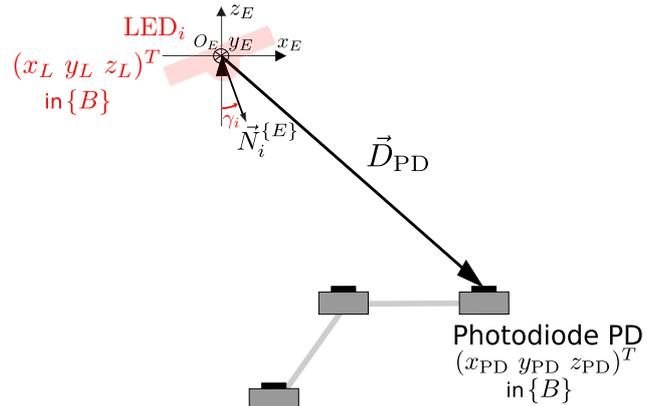
**FIGURE 18.** Illustration of the vector  $\vec{D}_{PD}$  with respect the coordinates of the LED<sub>*i*</sub> and the photodiode PD in  $\{B\}$ .
