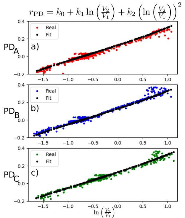
**FIGURE 11.** Plots of the sensor calibration results. The plots a), b) and c) define the calibration functions in black for the estimations of the heading and the robot's position along the  $x$ -axis.
