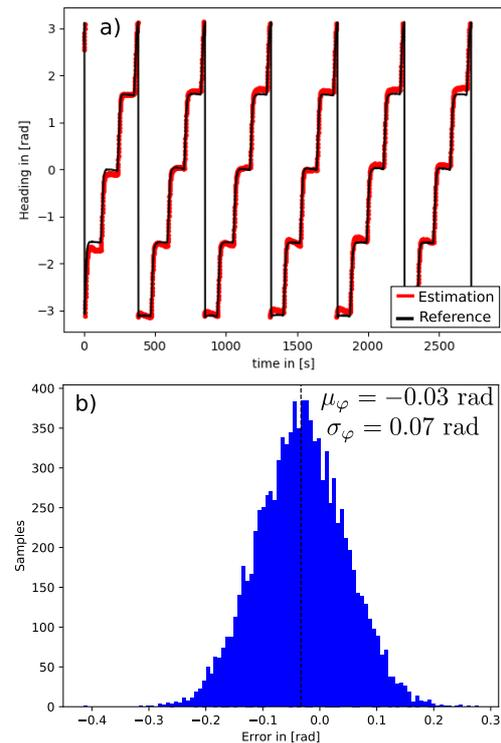
**FIGURE 14.** Estimation of the heading. a) Comparison of the heading estimation (in red) to the actual heading of the robot (in black) versus time. b) Histogram of the localization error in 2D using InLock sensor.
