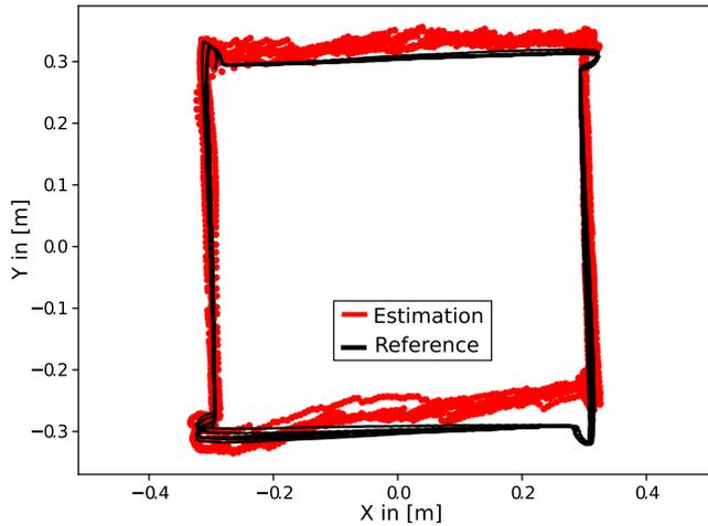
**FIGURE 17.** Comparison in 2D of the actual robot's trajectory (in black) to the position estimation (in red). The trajectory is repeated ten times. The robot's position is robustly estimated without drift by using the optical InLock sensor.
