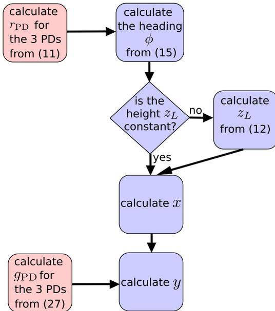
FIGURE 13. The algorithm flowchart describes the calculation of the heading and the positions in x and y of the mobile robot.
