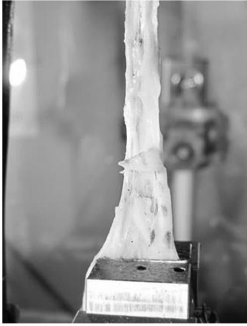
Figure 1: outer layer damage during an uniaxial dynamic tensile load of a human colon.
