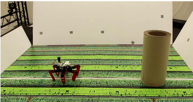
Fig. 5. The AntBot robot is walking straight forward in the direction of the obstacle (i.e. cylinder).
