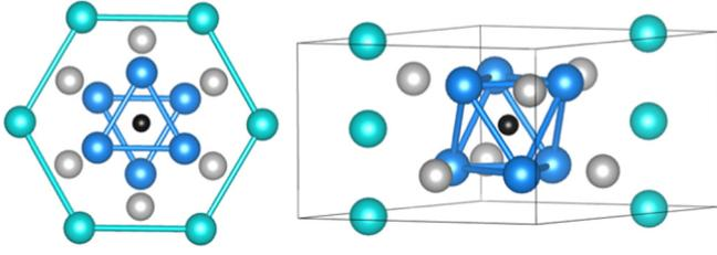
FIG. 1. Crystal structure of  $\text{Mn}_5\text{Ge}_3\text{C}$ . Left: Top view on the hexagonal plane; right: Side view. Colored spheres denote, respectively:  $\text{Mn}_I$  (green),  $\text{Mn}_{II}$  (blue), Ge (gray), and C (black). This drawing was prepared using the VESTA software [13].
