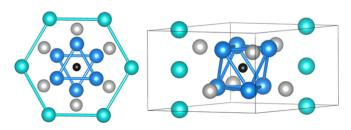
FIG. 1. Crystal structure of  $Mn_5Ge_3C$ . Left: Top view on the hexagonal plane; right: Side view. Colored spheres denote, respectively:  $Mn_I$  (green),  $Mn_{II}$  (blue), Ge (gray), and C (black). This drawing was prepared using the VESTA software [13].
