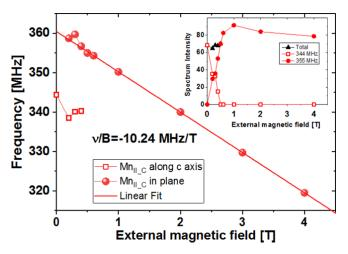
FIG. 10.  $^{55}$ Mn NMR frequency of the two components of NMR spectrum from the Mn $_{II\_C}$  sites of the Mn $_{5}$ Ge $_{3}$ C $_{0.2}$  film as a function of the in-plane field. Open squares: NMR signal along the c axis, spheres: NMR signal on the hexagonal plane. The inset: Intensities of the respective spectrum components as a function of the in-plane field strength and the total spectrum intensity (triangles) before the in-plane saturation.
