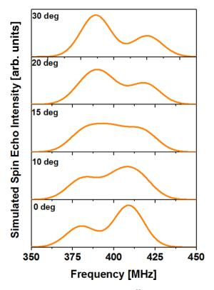
FIG. 7. The theoretical shape of the  $^{55}$ Mn NMR spectra from the  $Mn_{II}$  sites in the  $Mn_5Ge_3C_{0.2}$  film computed for the magnetic field of 4 T at various in-plane orientations with respect to the [010] direction.
