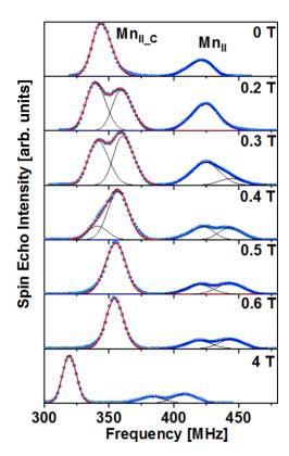
FIG. 4.  $^{55}$ Mn NMR spectra recorded at 4.2 K from the Mn<sub>II</sub> sites in the Mn<sub>5</sub>Ge<sub>3</sub>C<sub>0.2</sub> film at different values of the in-plane magnetic field. For details of spectrum decomposition, see the text.
