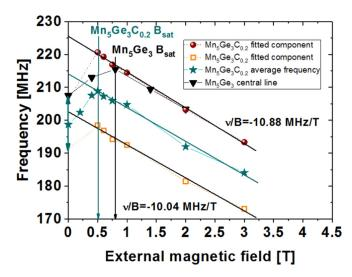
FIG. 12. Green stars: Central frequency of the experimental  $^{55}$ Mn NMR spectrum from the Mn $_I$  sites in the Mn $_5$ Ge $_3$ C $_{0.2}$  film (computed as a line first moment). Brown spheres and orange squares: Spectrum components identified in Fig. 11; black triangles: Central line of the Mn $_I$  quadrupolar quintet in the reference pristine Mn $_5$ Ge $_3$ . All plotted as a function of the in-plane magnetic-field strength.
