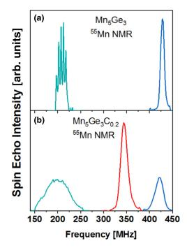
FIG. 2. Zero-field  $^{55}$ Mn NMR spectra recorded at 4.2 K from the 300-nm films of  $Mn_5Ge_3$  and  $Mn_5Ge_3C_{0.2}$  epitaxially grown on the Ge(111) substrate. Green: The NMR line from the  $Mn_I$  sites; blue:  $Mn_{II}$  sites with no carbon nearest neighbors; and red:  $Mn_{II}$  sites having carbon nearest neighbors.
