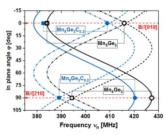
FIG. 8. Frequency branches of the NMR spectrum computed for three nonequivalent  $Mn_{II}$  positions (solid line denotes n=1, dashed line denotes n=2, dashed dot line denotes n=3) as a function of orientation of the in-plane field in  $Mn_5Ge_3C_{0.2}$  (blue lines) and in the reference pristine  $Mn_5Ge_3$  film (black lines):  $\nu_n(\phi) = \nu_{\parallel} + \Delta \nu \sin^2[\phi + (n-1)60] - \gamma B_{\rm ext}$ .
