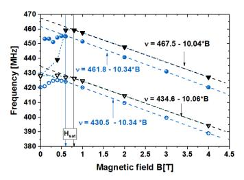
FIG. 9. NMR frequency of the two components of the  $^{55}$ Mn NMR line from the  $Mn_{II}$  sites not having carbon nearest neighbors, observed at  $\phi = 90^{\circ}$  in  $Mn_5Ge_3C_{0.2}$  (blue spheres) and in the reference pristine  $Mn_5Ge_3$  film (black triangles), plotted as a function of the in-plane field strength.
