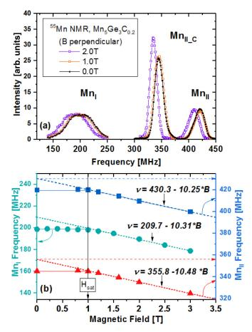
FIG. 3. (a)  $^{55}$ Mn NMR spectra recorded at 4.2 K from the Mn<sub>5</sub>Ge<sub>3</sub>C<sub>0.2</sub> film at different values of the external magnetic field oriented perpendicular to the film plane; (b)  $^{55}$ Mn NMR frequency in Mn<sub>5</sub>Ge<sub>3</sub>C<sub>0.2</sub> as a function of the out-of-plane field: Left scale: Mn<sub>I</sub> crystalline sites; right scale: Mn<sub>II</sub> crystalline sites. The colors of the symbols correspond to particular NMR lines as defined in Fig. 2.
