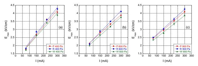
Figure 6: Maximum E-field strength ( $E_{max}$ ) obtained via the parabolic fit (red), Rickard model (blue) and Wroński model, vs. the discharge current, with pressures of 400 Pa (a), 600 Pa (b) and 900 Pa (c). The error bars are provided by the different fits.
