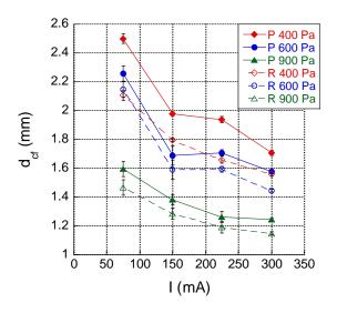
Figure 3: Comparison of the length of the cathode fall region vs. the discharge current, obtained with the parabolic fit (solid lines) and via the Rickards' model (dashed lines). Each pressure is represented by a different colour: 400 Pa (red), 600 Pa (blue) and 900 Pa (green). The error bars are provided by the fit.
