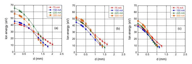
Figure 7: Ion energy in the cathode fall region vs. the distance from the cathode surface, discharge with with pressures of 400 Pa (a), 600 Pa (b) and 900 Pa (c) and four different currents (75, 15, 225 and 300 mA) obtained by the Wroński model. The error bars are provided by the fit.
