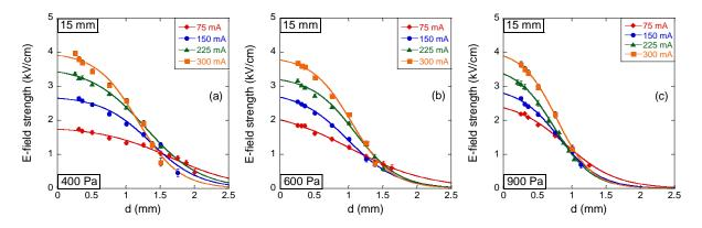
Figure 5: E-field strengths fitted with Wroński's model vs. the distance from the cathode surface, for four different currents values (75, 150, 225 and 300 mA), with pressures of 400 Pa (a), 600 Pa (b) and 900 Pa (c). The error bars are the same that in [20], uncertainties in the determination of the E-field.
