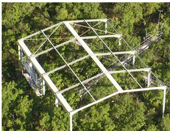
Figure 1. Oak Observatory of the Observatoire de Haute-Provence (O 3 HP). 43°56′06.74″ N, 5°42′38.57″ E. Rain exclusion device and the scaffolding for canopy measurements.
