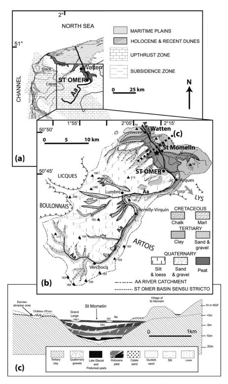
**Figure 1** (a) Location of the St-Omer basin (northern France). (b) Drainage basin of the river Aa and coring site (black star). The St-Omer basin *sensu stricto* is delimited by a dotted line. (c) Lithology of the St-Omer basin cross-section at St-Momelin (Gandouin, 2003)
