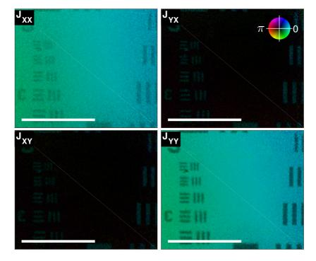
**Fig. S3.** Reconstructed Jones matrix maps of the scanned object, after data processing of the multicore fiber exit field. The corresponding reconstructed field is shown in Fig. 6. The Inset shows the complex value color coding, with phase encoded as hue and modulus as brightness. Scale bars are 100  $\mu$ m.
