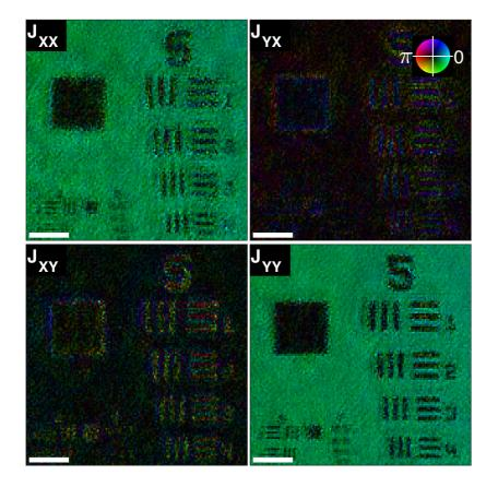
**Fig. S1.** Reconstructed Jones matrix maps of the scanned object, after data processing of the phase vortex beam. The corresponding reconstructed beam is shown in Fig. 4. The Inset shows the complex value color coding, with phase encoded as hue and modulus as brightness. Scale bars are 100  $\mu$ m.
