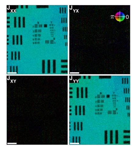
**Fig. S2.** Reconstructed Jones matrix maps of the scanned object, after data processing of the vectorial speckle. The corresponding reconstructed beam is shown in Fig. 5. The Inset shows the complex value color coding, with phase encoded as hue and modulus as brightness. Scale bars are 100  $\mu$ m.
