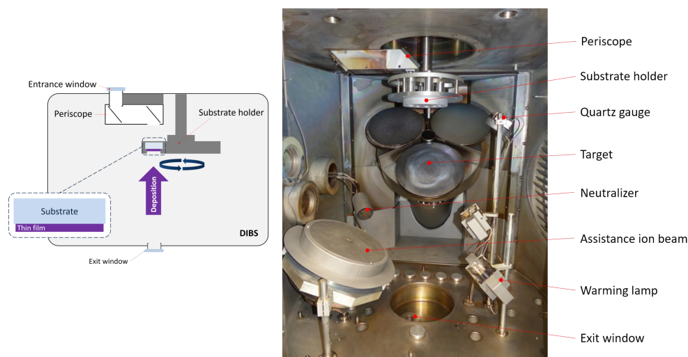
Fig. 1. The DIBS deposition machine (on the left, schematic view of the substrate configuration; on the right, picture of the inside of the machine).
