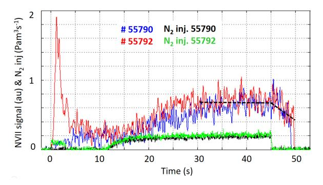
Time evolution of the Mass 28 ( $N_2$ ) recorded by the RGA in the mid-plane for the series of discharges (plasma from 0 to 50s range, except for # 55794 from 0 to 35s). The increase in the mass 28 signal with increasing discharge number can be attributed to the stronger seeding, but for the last pulse (# 55794) of this series, strong MHD activity occurred that could also explain the higher recovery due to different/enhanced plasma wall interaction with the potential  $N_2$  reservoir.
