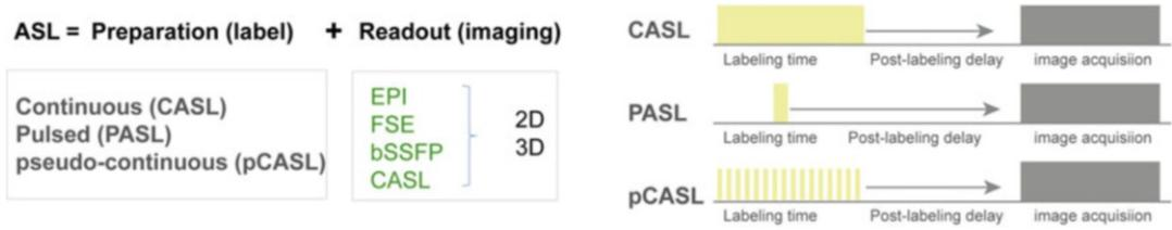
**Fig. 1** Left: All ASL pulse sequences consist of two modules: a preparation module to magnetically label flowing blood, and a readout module to generate paired images. Right: Schematic showing different labeling modules. A single or a train of radiofrequency pulse for labeling followed by a postlabel delay before the image is acquired within one TR.
