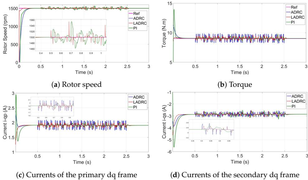
Figure 8. PMSM performance in the second faulty mode.
