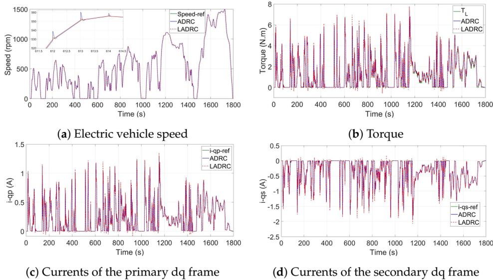
Figure 9. PMSM performance under WLTP drive cycle.
