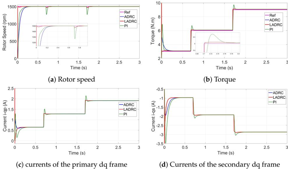
Figure 4. PMSM performance with load torque variation.
