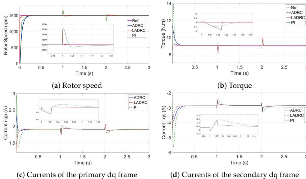
Figure 7. PMSM performance in the first faulty mode.
