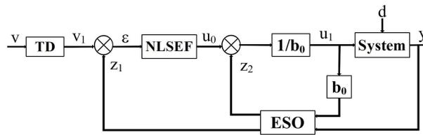
Figure 2. Schematic diagram of standard ADRC controller.
