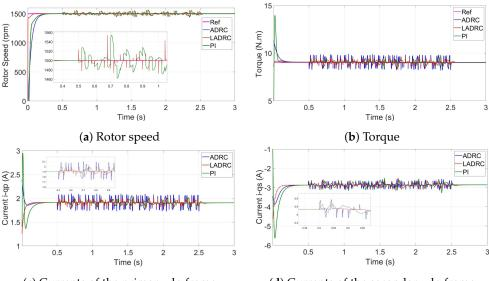
(c) Currents of the primary dq frame(d) Currents of the secondary dq frameFigure 8. PMSM performance in the second faulty mode.
