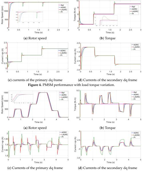
Figure 5. PMSM performance with speed variation.
