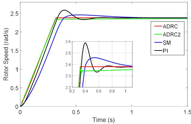
Fig. 6. Speed tracking comparison during starting stage.
