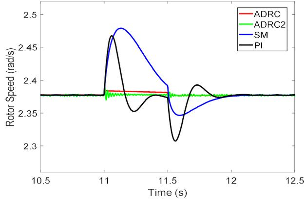
Fig. 8. Speed tracking comparison during turbine torque disturbance.
