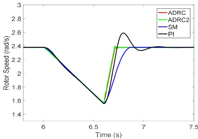
Fig. 7. Speed tracking comparison during current velocity disturbance.
