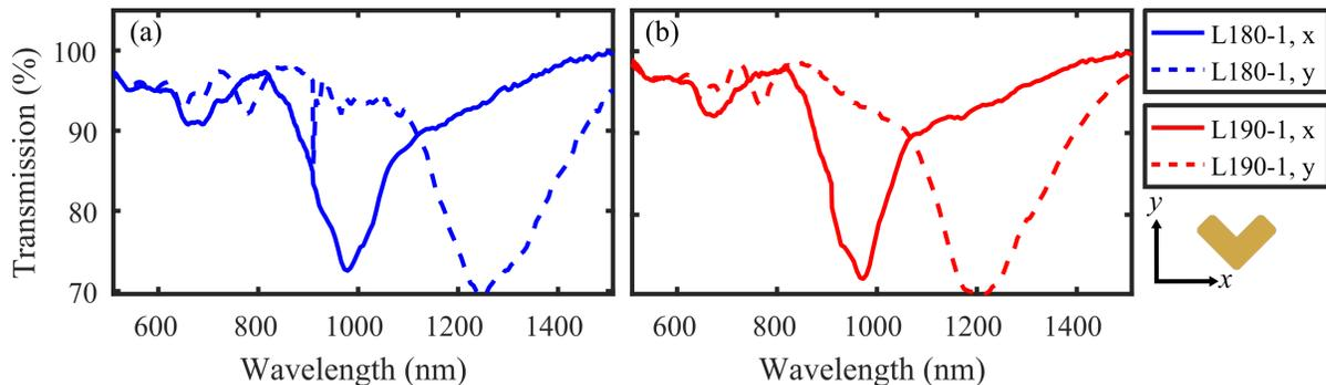
FIG. S1. Transmission spectra of single layer devices (a) L180-1 (blue) and (b) L190-1 (red). Broad plasmon resonances are visible near 970 nm and 1200 nm for  $y$ -polarized (dashed) and  $x$ -polarized (solid) light, respectively.
