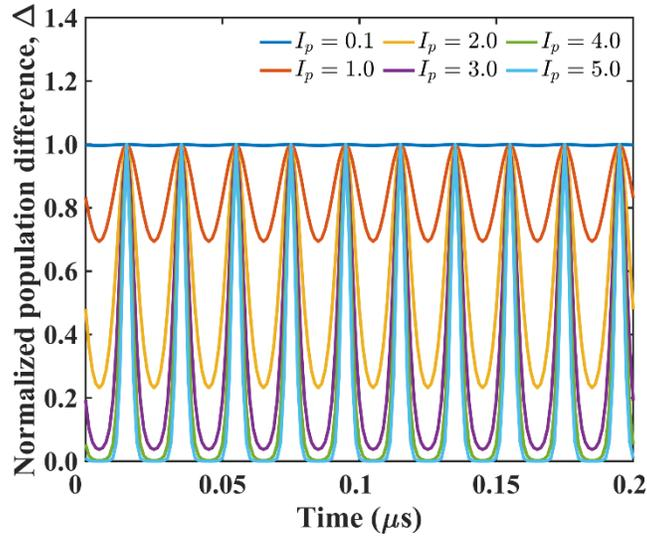
**Figure 3.** The effect on the population difference due to the modulation of the pump beam, at various intensities of the pump beam, for MSB. The intensity of the pump beam is given in multiples of 2.8 MW/cm<sup>2</sup>. The intensity of the Stokes beam was fixed at 1.6 MW/cm<sup>2</sup>. The
