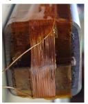
Fig. 1. MAG42-2, cross section of tested samples. 486 strands of 0.81 mm of diameter, with 324 of superconducting strands. Without (left) and with (right) the wound measurement pick-up coil.
