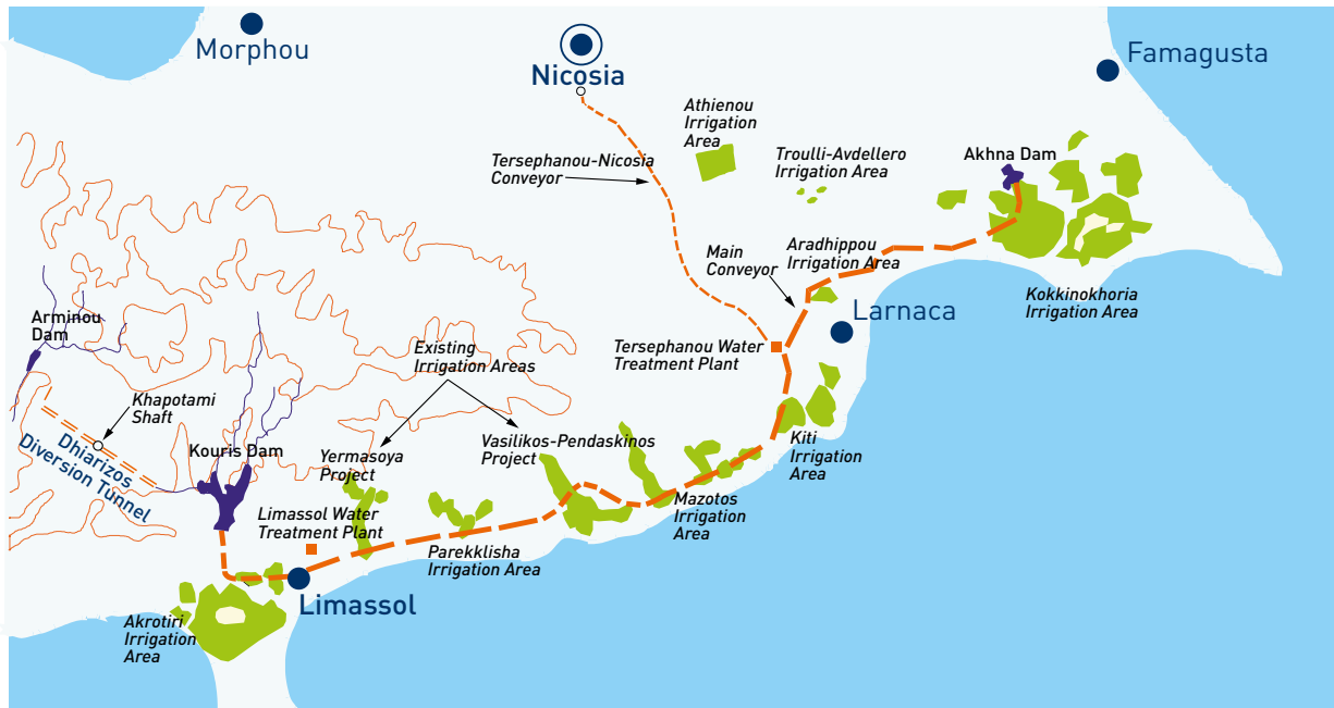
Figure 3.9 | Example for a large-scale IBT project is the Southern Conveyor Project on the island of Cyprus (Water Development Department Cyprus 2000).
