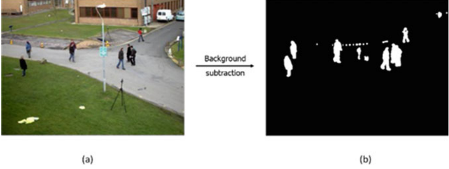
Fig. 2 Motion detection: a original image and b moving parts
