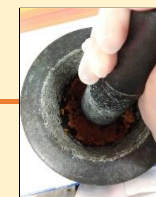
Laboratory scale extraction: Grinding of 15 ± 2 g of dry nuts, maceration with EtOAc (ethyl acetate), sonication and drying
