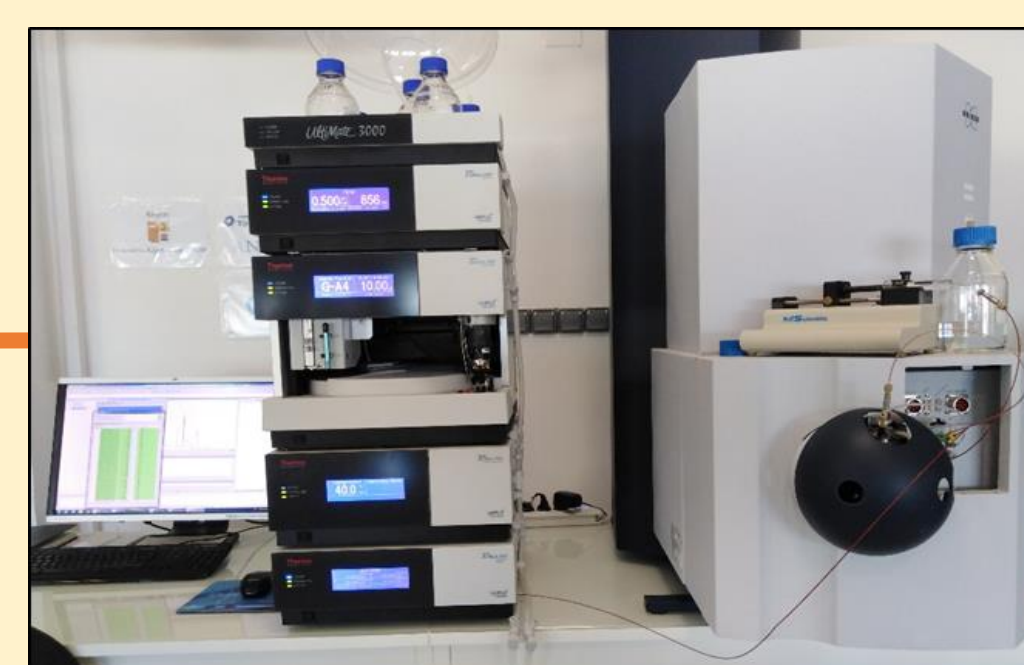
≈ 135 resinoid extracts analyzed in French Polynesia (LC-DAD, Luna C18 (250 x 4.6 mm, 3 μm)) and Marseille (UPLC-QqToF- MS/MS, Luna C18 (150 x 2.1 mm, 1.6 μm))
