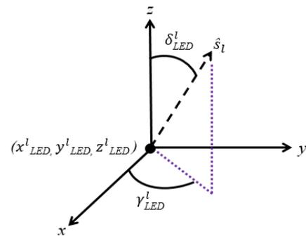
FIGURE 2. The orientation of  $l^{th}$  LED.
