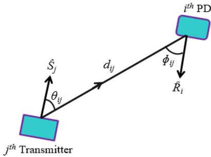
FIGURE 3. The LOS channel link between  $j^{th}$  transmitter and  $i^{th}$  PD.
