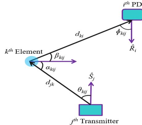
FIGURE 4. The NLOS channel link between  $j^{th}$  user and  $i^{th}$  PD reflected by the  $k^{th}$  element.
