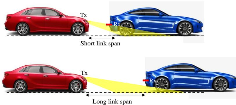
Fig. 9: V-VeLC links using HLs as the Tx's
