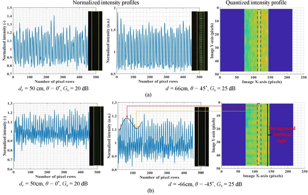
**Fig. 4.** Examples of captured illuminating POF at: (a)  $f_s = 300$  Hz and  $t_F = 200$   $\mu$ s, and (b)  $f_s = 500$  Hz and  $t_F = 400$   $\mu$ s. Note, yellow and red arrows highlight the intensity variations due to background ambient light.
