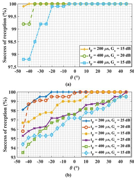
**Fig. 5.** Performance of OF-OCC: the success of reception with respect to  $\theta$  for  $f_s$  of: (a) 300 Hz, and (b) 500 Hz.
