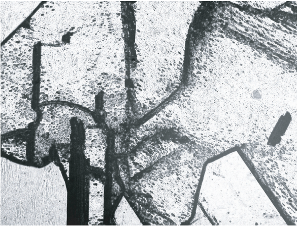
Fig. 5. Optical microphotography of the central part of Figure 3 sample after chemical etching. The lower values, 60 \mu\text{s} for \tau_p and 180 \mu\text{m} for L_p , are found in regions where the dislocation density is higher than 10^6 \text{ cm}^{-2} .
