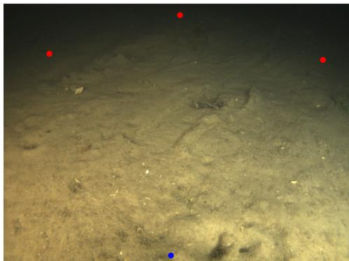
Figure 5. An example of underwater image showing minimum disparity (red dots, ~ 140 pixels) and maximum disparity (blue dot, ~ 430 pixels). Photograph COMEX ©.
