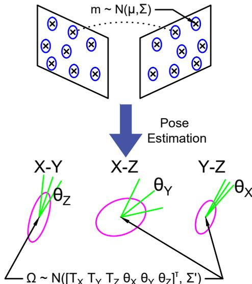
Figure 9. Illustration of error propagation through the pose estimation procedure. Estimated pose uncertainty is shown for each of the 6 DOF. Full covariance matrix can result from diagonal error distribution of matched 2D feature points
