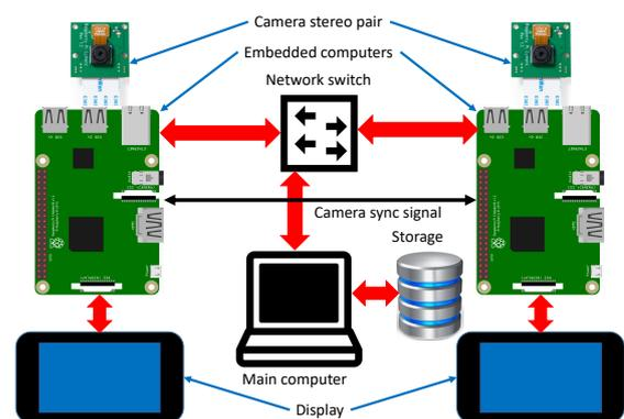
Figure 2. The built system internal design, it is composed mainly of (1) stereo camera pair, (2) Raspberry Pi © computers and (3) monitors.
