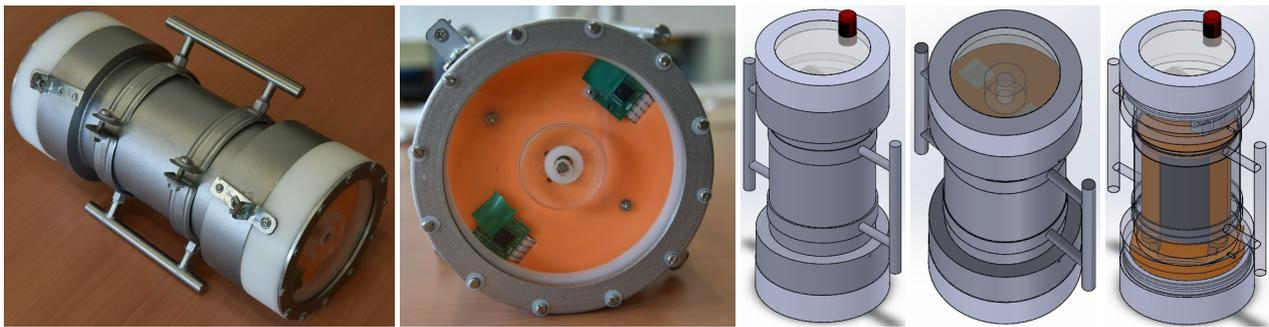
Figure 1. The built system prototype and design sketches.
