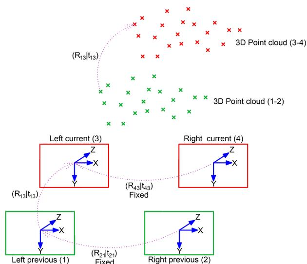
Figure 8. Image quadruplet, current (left and right) and previous (left and right) frames are used to compute two 3D point clouds. The transformation between the two points clouds is equal to the relative motion between the two camera positions.
