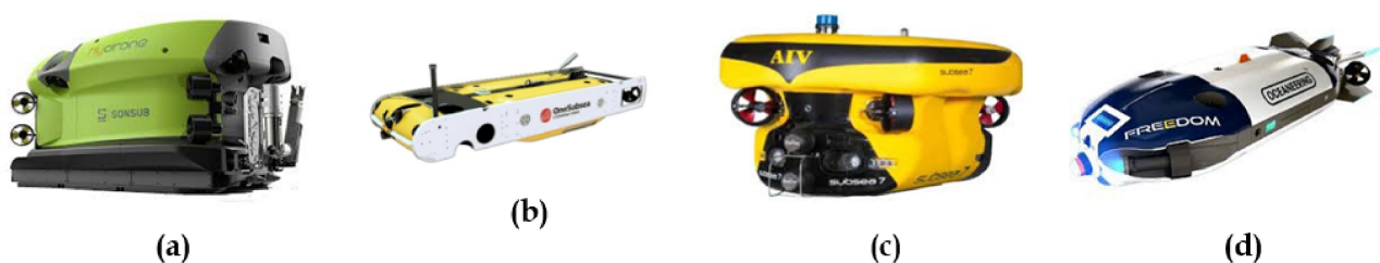
Figure 5. Some examples of Seabed-Hosted Vehicles (SHVs): (a) SAIPEM Hydrone-R [87]; (b) One-Subsea and SAAB Sabertooth [89]; (c) Subsea-7 AIV [86]; and (d) Oceaneering Freedom ROV [88].
