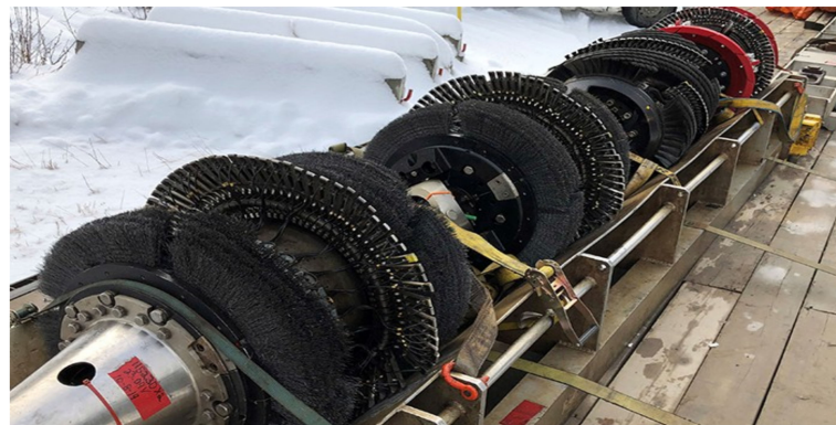
Figure 3. In-line Inspection tool from T.D. Williamson ( https://www.tdwilliamson.com/solutionspipeline-integrity/in-line-inspection (accessed on 9 July 2021)).
