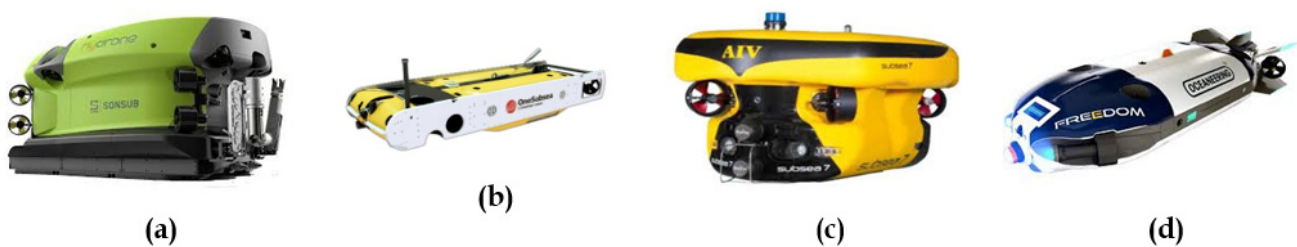
Figure 5. Some examples of Seabed-Hosted Vehicles (SHVs): (a) SAIPEM Hydrone-R [87]; (b) One-Subsea and SAAM Sabertooth [89]; (c) Subsea-7 AIV [86]; and (d) Oceanering Freedom ROV [88].
