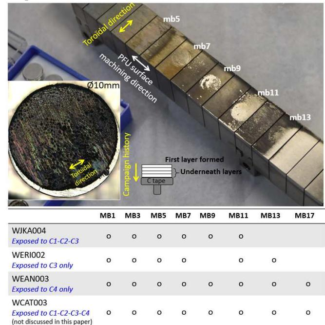
**Figure 3: Photograph of PFU WEAN003 taken after the deposits have been collected using the SEM holder. Inset showing a photograph of the SEM sample holder with the deposit on the carbon tape. The table below details the MB’s where deposits have been collected for each PFU.**
