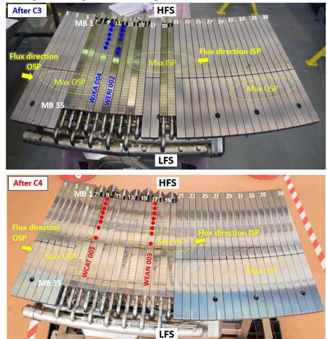
**Figure 2: Configuration of the WEST test divertor sector for the C3 campaign with 12 ITER like PFU (top) and for the C4 campaign with 14 ITER like PFU (bottom). The PFU numbering on the sector (from 1 to 38) is indicated as well as the PFUs where the deposits have been collected after the C3 and C4 campaigns. Finally the areas of maximum plasma loads alternating on the HFS (max ISP) and LFS (max OSP) due to the impact of the magnetic ripple are shown.**
