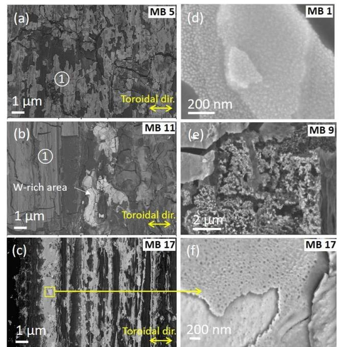
**Figure 5:** SEM images (BSE mode) showing the morphology of the deposits collected after the C4 campaign on WEAN003 (a) MB 5 (b) MB 11 and (c) MB 17. On the right hand side, high magnification images of (d) nanoparticles found in the first layer of MB 1, (e) particles in the underneath layer of MB 9 (f) nano-holes in a W-rich layer of MB 17.
