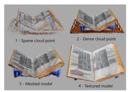
FIGURE 12.4 STEPS OF THE 3D DIGITZATION F A MANUSCRIPT, A GLOSSED LATIN BIBLE (ESTIMATED FOURTEENTH CENTURY) (C) MARSEILLE, BMVR, MS. 11, F. 31V-32R; IMAGES PREPARED BY LÉO PASCAL. WE ALSO THANK THE CURATOR OF THE BMVR ALCAZAR LIBRARY OF MARSEILLES, SOPHIE ASTIER.
