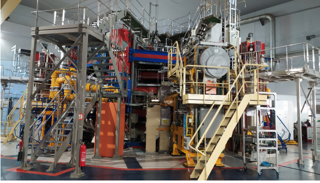
Fig. 2. General view of the WEST tokamak and the experimental hall. The support of the RTSER bench is visible at the bottom right of the image, partially behind the gateway stair.
