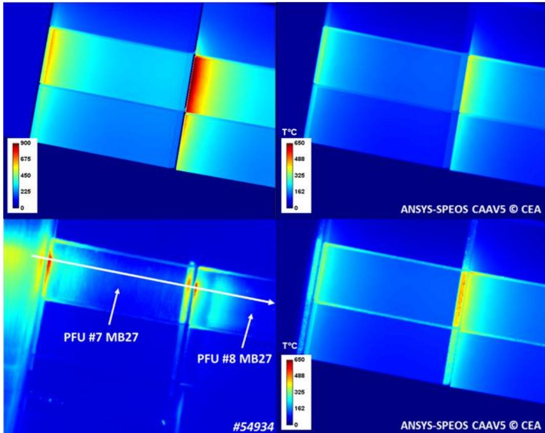
Figure 13 Three steps of the ANSYS-SPEOS simulations that give synthetic data base on IO modeling taking into account: the optical blurring (top left panel), the isotropic emissivity spatially uniform on surfaces (top right panel), and the complex model reflectance with Lambertian emission: 40% diffuse and 60% specular (bottom right panel), are compared to the VHR IR data (bottom left panel).
