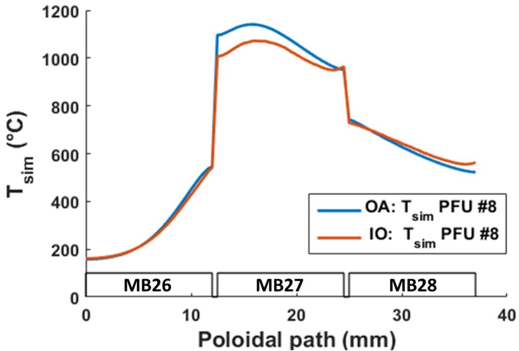
Figure 12 Poloidal profiles of the PFU #8 based on FGB measurements ( $71\text{MW}\cdot\text{m}^{-2}$ ,  $\lambda_q = 18\text{ mm}$  and  $S = 5\text{ mm}$ ), obtained through 3D FEM modeling based on OA (blue) and IO (red) heat flux modeling.
