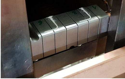
Figure 2: Seven actively cooled monoblocks (numbered from 1 to 7 from right to left) facing the electron beam gun of HELCZA HHF facility and framed by movable shielding screens. An empty lateral groove located at 5 mm beneath the surface exposed to heat flux is visible on the monoblock 4 (central). The paths of the two thermocouples wires running across monoblocks 2-3 and 5-6 are visible through the white marking of the glue. The probing spots of the thermocouples are located respectively on monoblocks 3 and 6 at 5 mm beneath the exposed surface.
