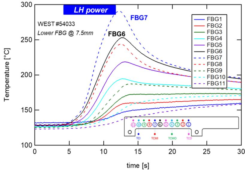
Figure 3: FBG temperature measurement during WEST experiment #54033 ( $I_p = 500$  kA,  $P^{LH} = 4.5$  MW) showing the temperature rise and cooling of the tile during and after the power cut-off respectively.
