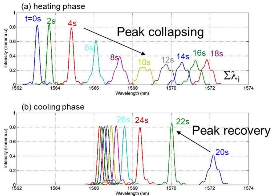
Figure 7: Spectrum of the Bragg peak FBG#8 at different time step (#55070). During heating phase (a) exhibiting peak collapsing due to  $T^\circ$  gradient and followed by cooling phase (b) with peak recovery.
