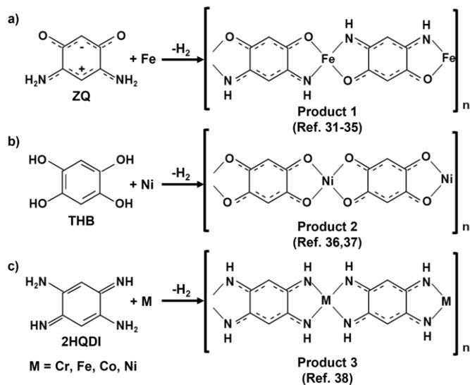
**Scheme 2** Schematic illustration of the 1D coordination reactions used for the synthesis of 1D-cMOFs on surfaces. (a) 1D-cMOF obtained from ZQ and Fe atoms. (b) 1D-cMOF from THB and Ni atoms. (c) 1D-cMOF obtained from 2HQDI and different metals (M=Cr, Fe, Co, Ni).
