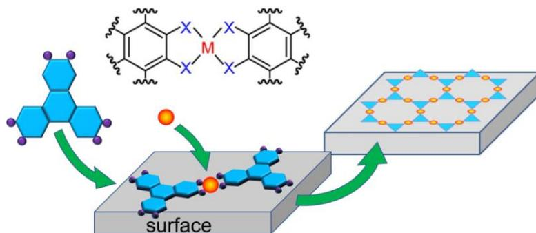
**Scheme 1** On-surface synthesis of single-layer 2D-cMOFs based on bis-(di-X)M coordination (X=thiol, hydroxyl, amino).
