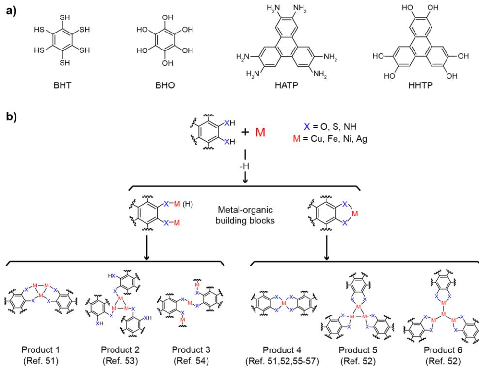
**Scheme 3** (a) Chemical structures of the molecular ligands used for preparation of 2D-cMOFs on surfaces. (b) Schematic illustration of the on-surface dehydrogenation coordination reactions and the structure of the products proposed in the corresponding works.
