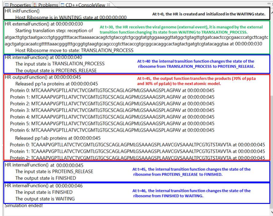
Figure 5: Simulation of the obtained DEVS model in the CD++Builder development environment.
