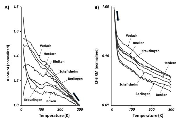
**Figure 12.** Magnetic results for Opalinus Clay. Cooling (**A**) and warming (**B**) of artificial remanence imparted at room temperature (RT-SIRM) and 10 K (LT-SIRM). The values of RT-SIRM and LT-SIRM were normalized. See Table 2 for the magnitude of the remanence.
