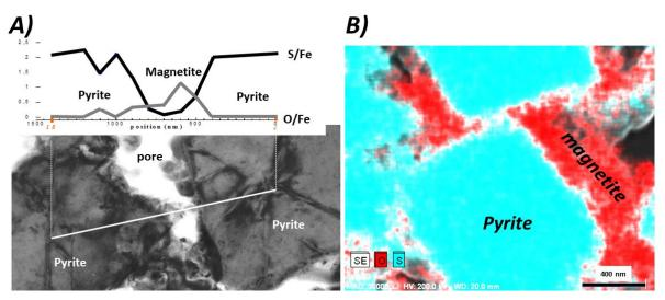
**Figure 10.** Transmitted electronic microscopy (TEM) microphotograph of pyrite from the FIB section (see Figure 9). (**A**) EDX profile between two pyrite grains. In between, iron oxide was detected. This was presumably magnetite. (**B**) EDX map of oxygen and sulfide. The pyrite grain was not oxidized, and iron oxide—presumably magnetite—framed the pyrite.
