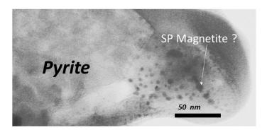
**Figure 11.** Transmitted electronic microscopy (TEM) microphotograph of pyrite framed by a gel in which nanometric euhedral crystals can be seen. These minerals were probably superparamagnetic (SP) magnetite.
