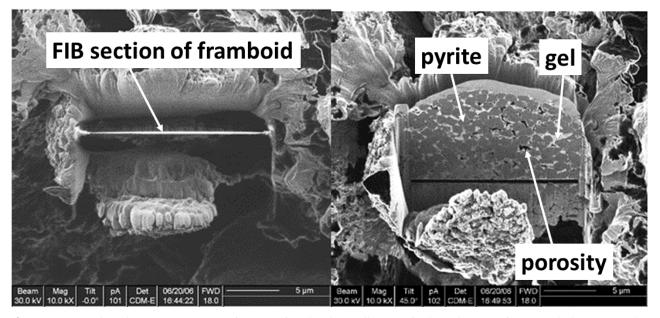
**Figure 9.** Focused ion beam (FIB) section of a pyrite framboid in Callovo-Oxfordian claystone from Borehole EST211. This sample was heated for 67 days at 95 °C. Lateral view (right) shows that pyrite (dark grey) is framed by a gel (light grey). Porosity (dark) is present within the framboids.
