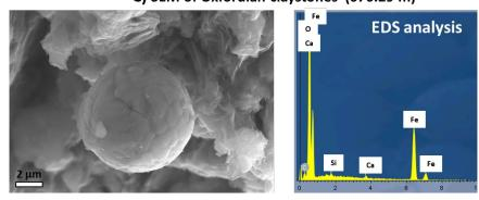
**Figure 8.** Scanning electron microscopy (SEM) observation of shales from Borehole EST433. Framboids of pyrite (**A**) and partially oxidized pyrite (**B**) observed in Toarcian claystones. (**C**) Spherule of former pyrite framboids oxidized observed in Oxfordian claystones and the EDS analysis.
