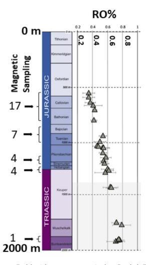
**Figure 4.** Peak burial temperature proxies from Borehole EST433. The reflectance of vitrinite (RO%) from ~0.3 to ~0.8 indicated that organic matter maturity was within the oil window. The numbers on the left refer to sampling for magnetic analysis. Data from Blaise et al. [8].
