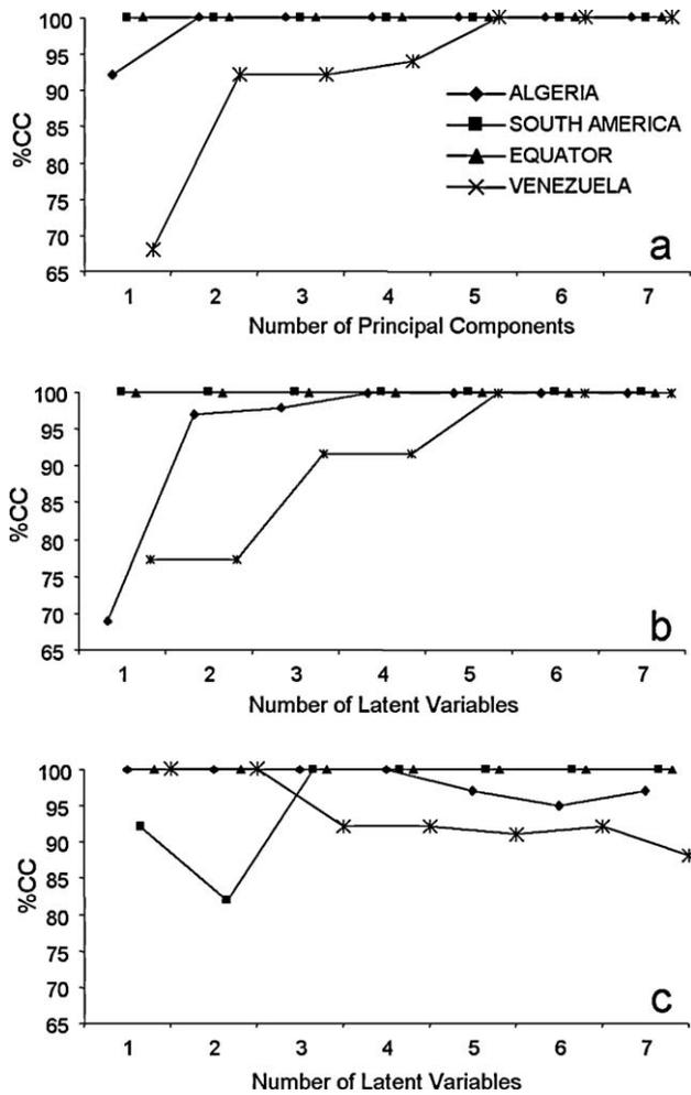
**Fig. 3.** Percentage of correct classification (%CC) for each petroleum oil origin as function of: (a) the number of principal component used in the SIMCA model; (b) the number of latent variable used in the PLS2-DA model; (c) the number of latent variable used in the PLS1-DA model.
