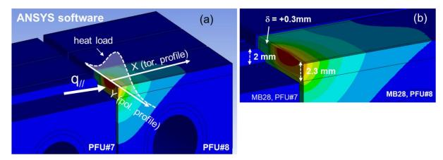
Figure 2: Thermal modelling assuming  $q_{//=}$  107 MW.m<sup>-2</sup>,  $y_0$  = 4.2 mm;  $\lambda_q$  = 10 mm, S = 1 mm as depicted in equation (3). (a) full view showing the groove and the overexposed LE to be melt, (b) zoom on the overexposed sharp LE showing the vertical misalignment between PFU#7 and PFU#8.
