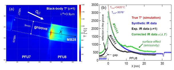
Figure 5: (a) VHR IR image during the melting experiment #56541 at t=8s when the thermal equilibrium is reached. (b) Temperature distribution along the toroidal direction: experimental IR data (black crosses), corrected (green crosses), synthetic (blue crosses) and FEM data (red line).
