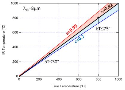
Figure 6: Error bar due to emissivity uncertainties for  $\lambda_{IR}=8\mu m$ . Lower and higher emissivity lead to under (blue) and over-estimation (red) of the true surface temperature.
