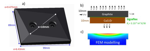
Figure 5: (a) CAD view of the graphite tile. 2D cross section of the assembly: (b) schematic picture of the assembly and (c) thermal modelling performed by CASTEM.
