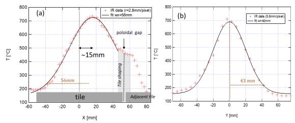
Figure 13: Horizontal (a) and vertical (b) temperature distribution extracted from IR movie at t=8s (#20181009.041,  $\theta$ =58°, 551 kW continuous). Experimental data are fitted with Gaussian function as given in equation 4. The shaped part of the tile is shown in blue as well as the poloidal gap (limit to the adjacent tile).
