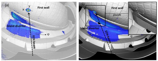
Figure 8: IR data during W7-X ECRH plasma experiment with shinethrough power hitting graphite tiles and CAD geometry of the inner wall in the scene model. (a) #20171121.13 with  $\theta$ =17° (775 kW modulation 5 Hz, duty cycle) and (b) #20181009.41 with  $\theta$ =58° (551 KW continuous heating)
