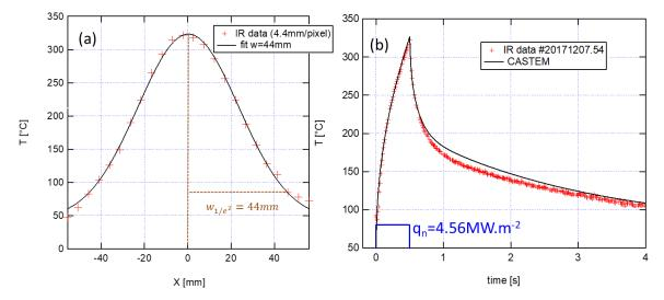
Figure 9: (a) Temperature distribution extracted from IR movie at t=0.5s (at the end of the EC shot). Experimental data are fitted with Gaussian function (equation 4). (b) Maximum temperature on the tile surface, IR measurement (red points) and CASTEM simulation (black line) after iterative loop.
