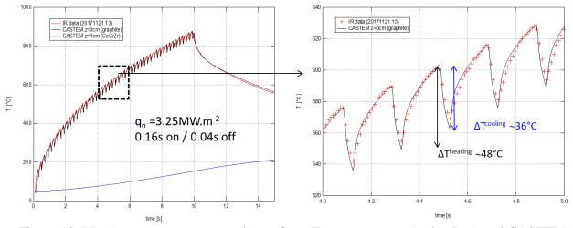
Figure 12: Maximum temperature on tile surface, IR measurement (red points) and CASTEM simulation (black and blue lines on top surface and CuCrZr interface respectively) after iterative loop (a) full pulse and (b) zoom over 5 periods
