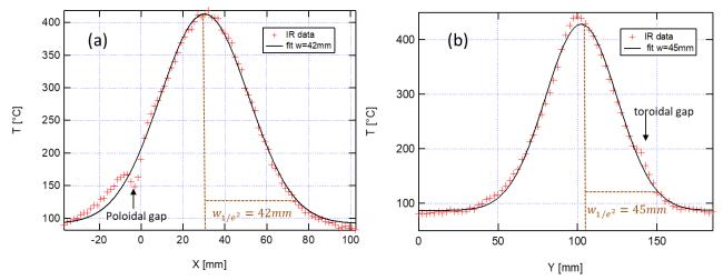
Figure 10: Horizontal (a) and vertical (b) temperature distribution extracted from IR movie at t=2s. Experimental data are fitted with Gaussian function as given in equation 4. The sides of the tile are spotted by the gaps between two neighboring tiles.
