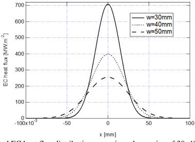
Figure 4: Simulated EC heat flux distribution assuming a beam size of 30, 40, 50 mm and 1MW power injected.
