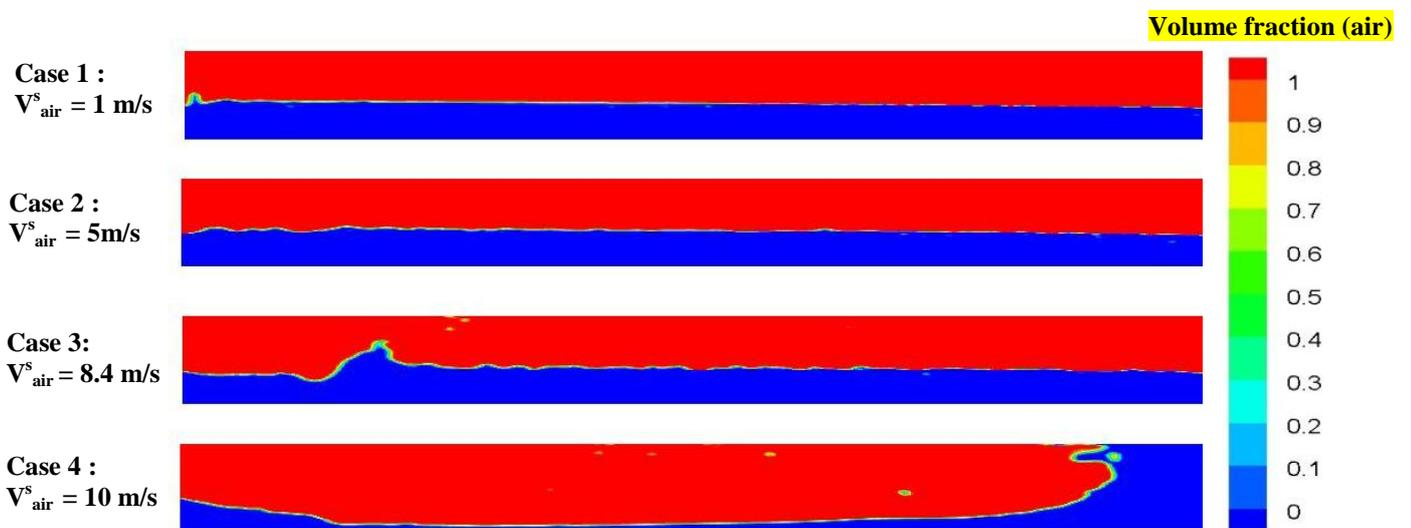
Fig.6: Contours of volume fraction in the median plane for air-water flow for different superficial air velocities at  $t = 0.4$  s
