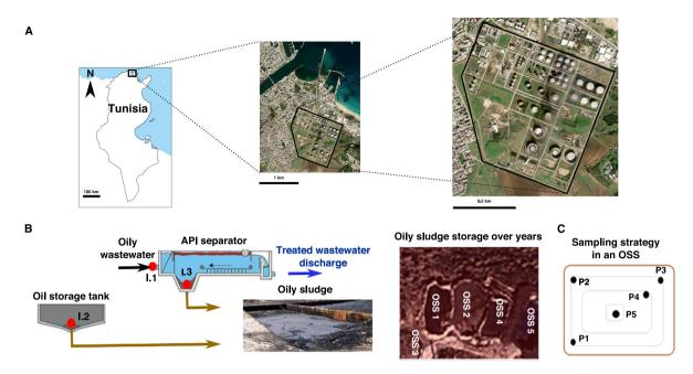
**Fig. 1.** Location of the Tunisian Company of Refining Industries STIR at Bizerte (A), schema of oily sludge (OS) generating process (B), and sampling strategy in oily sludge storage (C). The sites (I.1 to I.3) for sampling OS for bacterial isolation are indicated by red circles. OSS1 to OSS5: Oily Sludge Storage (OSS). P1 to P5: sampling sites in an OSS. Maps were generated using Plans (version 2.0).
