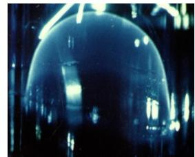
Propane flame propagating upwards
