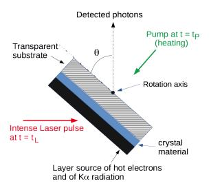
FIG. 10. Another possible experimental setup for pump-probe *Transmission* Kossel diffraction experiments.
