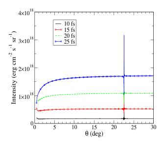
FIG. 3. Snapshots at different times of the  $K\alpha_1$  emission from a Ni sample as a function of the observation angle. Parameters of the simulation correspond to Fig. 2.
