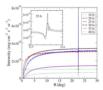
FIG. 4. Snapshots at different times of the  $K\alpha_1$  emission from a Ni sample as a function of the observation angle. Parameters of the simulation are given in the text. The inset is a zoom of the emission for the time of maximum emission. Dotted line is the broadened profile when one takes into account the FWHM energy broadening of the  $K\alpha_1$  line.
