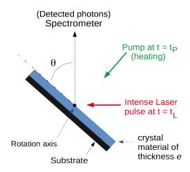
FIG. 9. Geometry of a possible experimental setup for pump-probe Kossel diffraction experiments.
