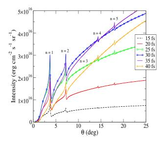
FIG. 7. Snapshots at different times of the Mg K $\alpha$  emission from a 1  $\mu$ m thick multilayer (Mg/Co)<sub>125</sub> as a function of the observation angle. Parameters of the simulation are given in the text. Kossel patterns are labeled by their Bragg order.
