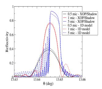
FIG. 1. Rocking curve of Ge 111 samples of different thicknesses around the Bragg angles at 8047.8 eV. Plain lines correspond to calculations based on the standard methods of the XOP package, <sup>32,33</sup> dashes: present 1D model as discussed in the text.
