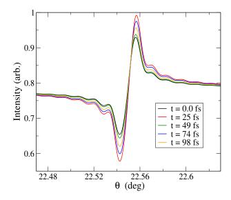
FIG. 8. Snapshots at different times during a phonon oscillation, of the  $K\alpha$  emission from a 400 nm thick Ni sample as a function of the observation angle around the Bragg angle. Parameters of the simulation are discussed in the text.
