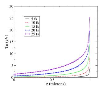
FIG. 2. Snapshots at different times of the thermal electron temperature in a 1  $\mu$ m thick Ni foil. The hot electron beam comes from the right. Parameters of the simulation are given in the text.
