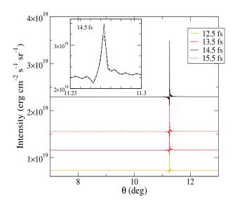
FIG. 6. Snapshots at different times of the  $K\alpha_1$  emission from a Mo sample as a function of the observation angle. Parameters of the simulation are given in the text. The inset is a zoom of the emission for the time of maximum emission. Dotted line is the broadened profile when one takes into account the FWHM energy broadening of the  $K\alpha_1$  line.
