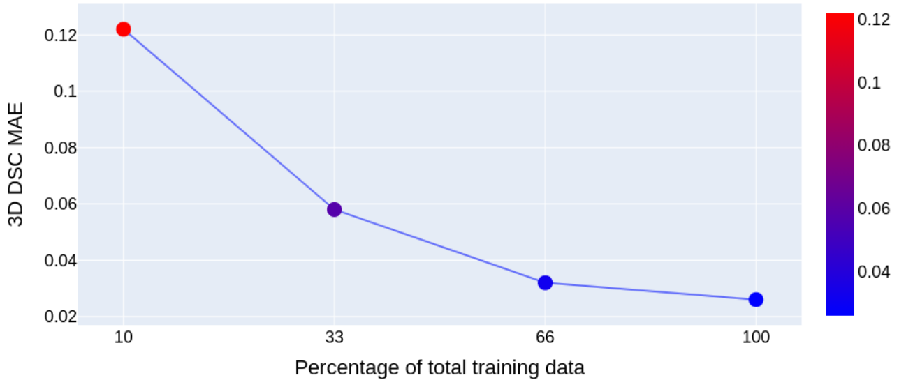
Fig. 8. 3D DSC MAE (averaged over all LV classes) as a function of the percentage of total training data used during training. The model used here is QC U-Net 2D_R .
