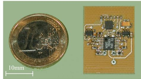
**Figure 2.** The μC-based EMD circuit is implemented on a 400μm-thickness PCB (size : 20×27mm, mass : 0.8g).
