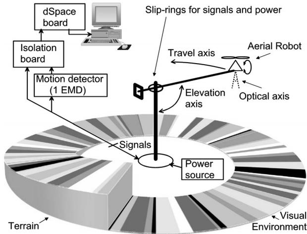
**Figure 3.** The test-rig is composed of a pantographic whirling arm supporting a MAV which flies over a 4.5-meter outside diameter arena. The textured environment below consists of randomly distributed, variously contrasting sectors.
